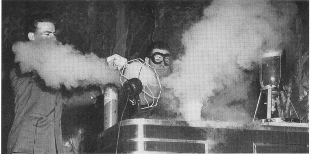
In the above spectacular experiment Mr. Hayes and Mr. Herron, directors of the exhibit, manufacture butyl rubber. The reaction takes place through the skillful juggling of carbon and hydrogen molecules spurred on by the catalyst—Boron trifluoride.
